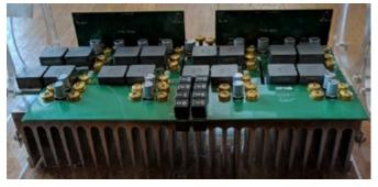
Figure 6: A 97% efficient 6 kW 48 V - 14 V bi-directional automotivegrade DC-DC buck/boost converter that uses 16 EPC2208 100 V eGaN FETs.
